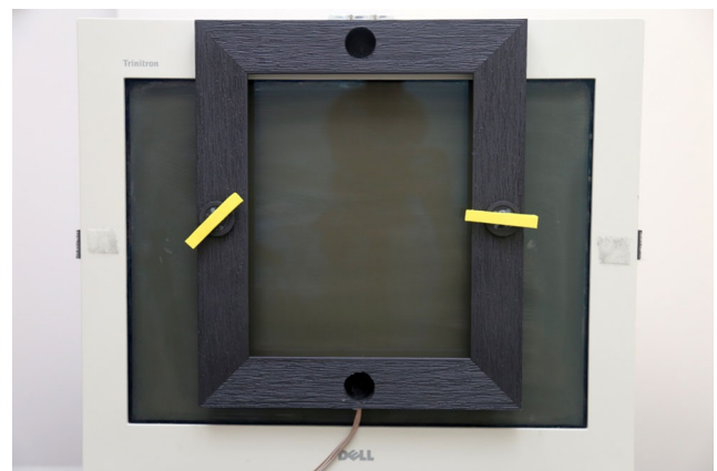
Fig. 4 Apparatus for Experiment 2. Each of two motors could rotate the yellow bars (clockwise) during the trials. The figure-eight placeholders, which changed to letters, appeared on the monitor adjacent to the yellow bars
